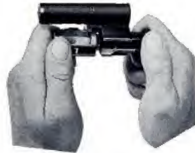
Fig. 34 Removing the bolt assembly components
